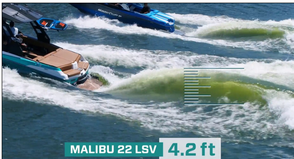
Figure 2-2. Malibu 22 LSV wave with factory ballast setup (Source: Guinn Partners 2019).
