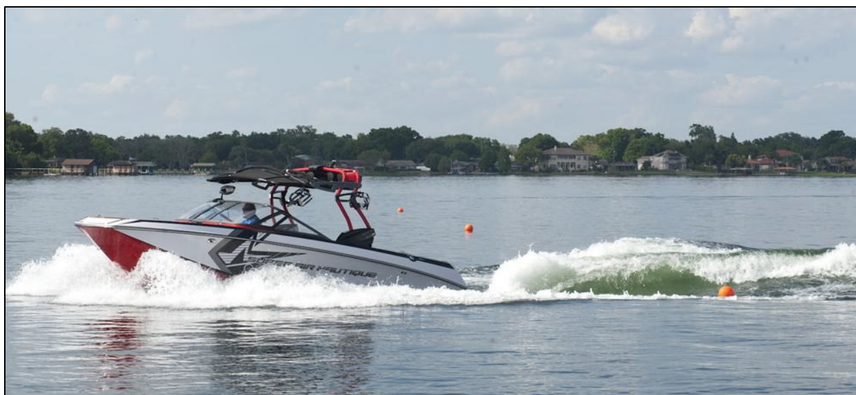
Figure 2-3. Nautique G-23 used during WSIA study operating under wakesurfing condition (Goudey and Girod 2015)
